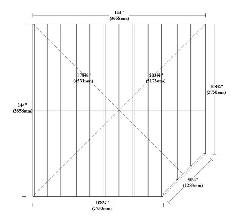
NB:- Floor joists run from right hand back to left hand front.
